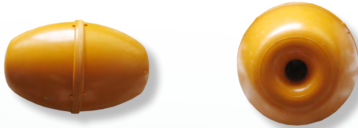
17 060 230 # 30G-2 ABS 200m WD 437mm x 290mm + 40ml Hole - 20kg buoyancy
